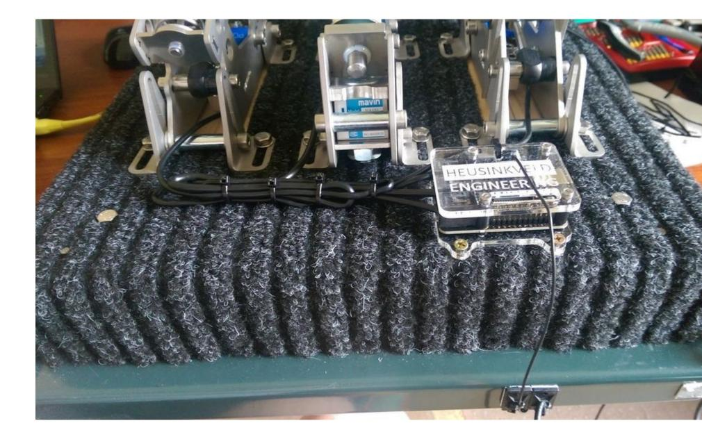
For the wheel controller, I run a simple Gnd cable from one of the ground pins on the button controller board, here I am using a BBI32, as an example, to a bolt on my QR1 quick release. Again, note you need to make contact with bare metal on the QR.....I use a simple spring washer underneath the lug, this will cut through the anodizing, but in any even, use a multimeter and test for continuity from your Gnd pin to the servo once the wheel is mounted to the servo.....
